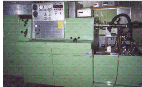
Figure 3. Test engine board for testing gear pumps.
