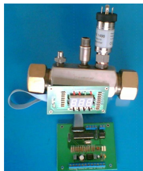
Fig.7. Mechatronic module for monitoring hydraulic parameters
