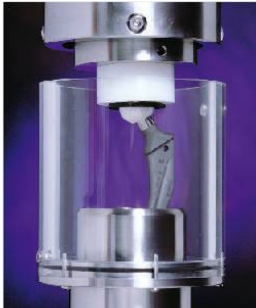
Figure 1 The specimen fixture for endurance properties determination
